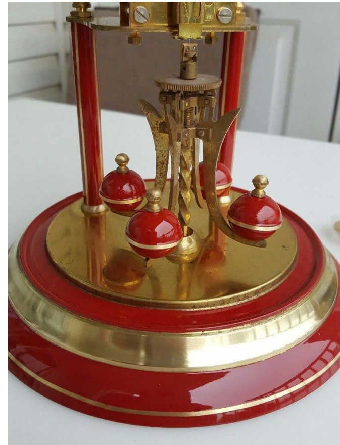
Figure 2: Torsional pendulum of Kundo 400 Day Anniversary Clock
